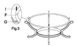
Step 4: Place the fire bowl (E), log grate (D), mesh cover(B) on the assembled base.
